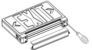
2.Knockout in back of mounting plate and push wires through the hole.
