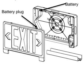
3.Connect the battery to battery plug.
